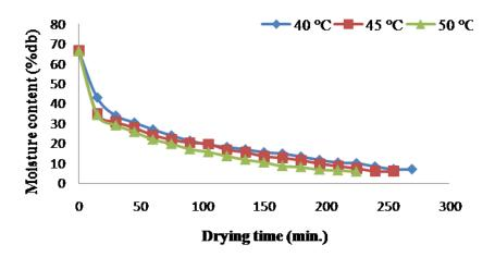
Fig. 3: Variation in moisture content (%d.b.) with drying time (min): fluidized bed drying
