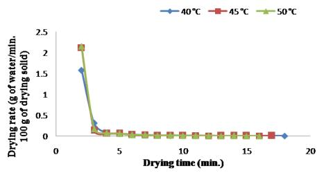
Fig. 4: Variation in drying rate with drying time (min): Fluidized bed drying
